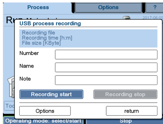
Fig. 23: Dialogue box "USB process recording"
