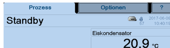
Fig. 39: Countdown of the password timer and the button with the lock symbol
